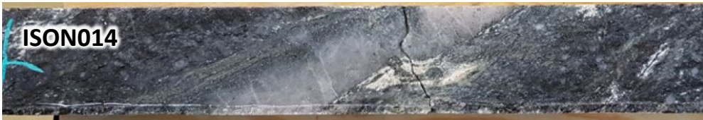
ISON014 162.56-163 m 18.1 g/t Au. Qtz vein in sheared feldspar amphibole porphyry
